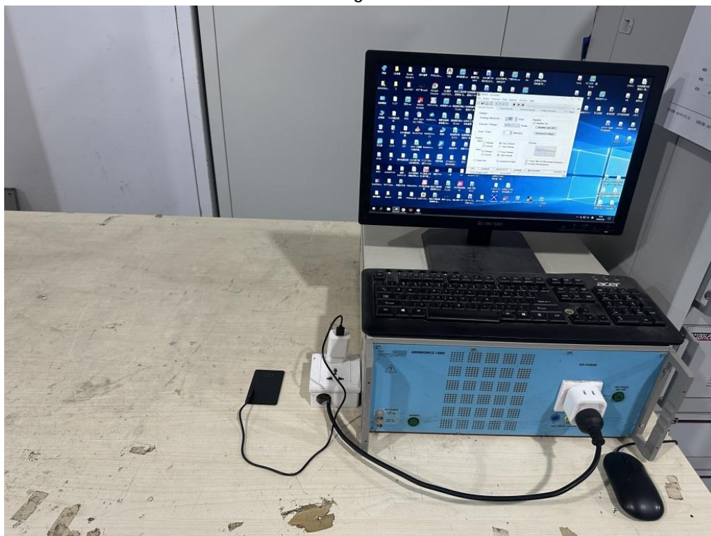
Harmonic Current/ Voltage Fluctuation and Flicker
